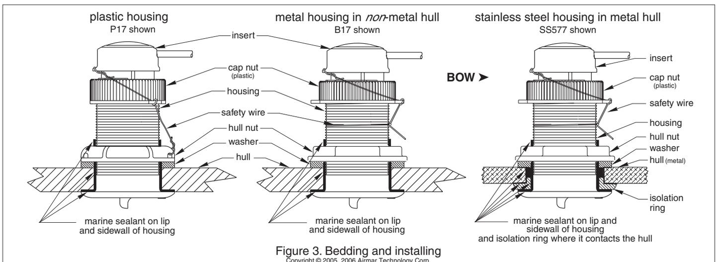
**Stainless steel housing in a metal hull**—To isolate the stainless steel housing from the metal hull, slide the isolation ring onto the housing. Apply *additional* sealant to the surfaces of the ring that will contact the hull, filling any cavities in and around the ring.
