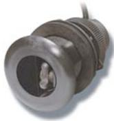
The industry's only depth, speed and temperature retractable transducer is now available with a valve! The DST800V meets customer demand for our patented valve assembly that prevents water from rushing into the hull when the insert is removed. And the addition of a valve lets boaters service the new DST800V while the vessel is in the water, saving time and money!
