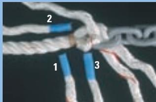
**Do the twist.** The strands tend to unravel a bit at this point so it is important, for neatness, to keep them tightly twisted.
