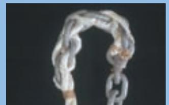
**Around the bend.** This elongated chain-to-warp splice is very flexible and goes through my chain-to-rope windlass with little or no trouble.
