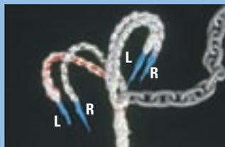
**In, then out.** Take a left pair and a right pair and thread it through the link. Then take the other left and right pairs and thread them through the link from the opposite direction over the top of the other two pairs.
