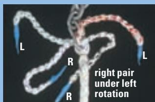
**Tunnel tricks.** Here's where it gets tricky. Turn the line so you can clearly see "the rotates to the left" weave on the body of the line. Take a right pair and slip it under the closest left-rotating pair. You may need to use a fid or a pencil to create this tunnel. Remember, right pairs slip under left pairs from right to left. You will notice that your tucked pair will have a partner weave that it travels along with.
