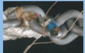
**Tie it off.** Using heavy waxed twine and a sail needle, tightly bind the ends to the chain links and then use the hot knife to cut off the excess. Keep the melted plastic ends as small as possible.
