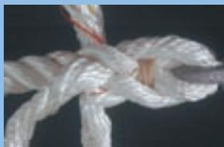
**Over under.** Take the Number 1 strand and go over one strand and then under the next strand. Do the same with Number 3. If you did it right, all three strands should appear to come out of the twisted rope at the same level but from between different strands. This is the most critical part of the splice. If you get this right, you are home free.
