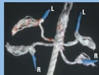
**Twist and shout.** You're almost there. Tuck the remains of each pair in the same pattern as before until there is only about an inch or so of strand poking out. Keep a twist on the remains of the strands.
