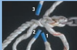
**Tuck away.** Do two complete tucks with all three strands, threading through against the wrap. Keep everything flowing in a counter twist pattern. Weave each over the next strand then under the one after that.
