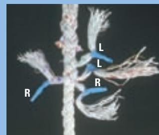
**Pull tight.** Once you have tucked as far as you can, pull the splice tight and then cut off the strands, leaving 1/4 to 1/2 inch sticking out.
