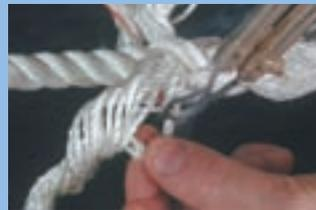
**Taper down.** After two tucks for each strand, take your hot knife and — from where the strand emerges from under a strand — cut off one third of the threads of each strand. Leave ½ inch or a bit more sticking
