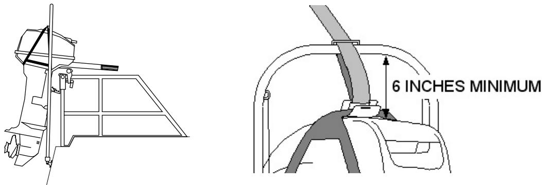
**IMPORTANT!** The frame must be mounted high enough to lift the motor clamp clear of the mounting bracket. This typically means leaving a MINIMUM of 6 inches from the bottom of the outboard carrying handle to the bottom of the frame.
