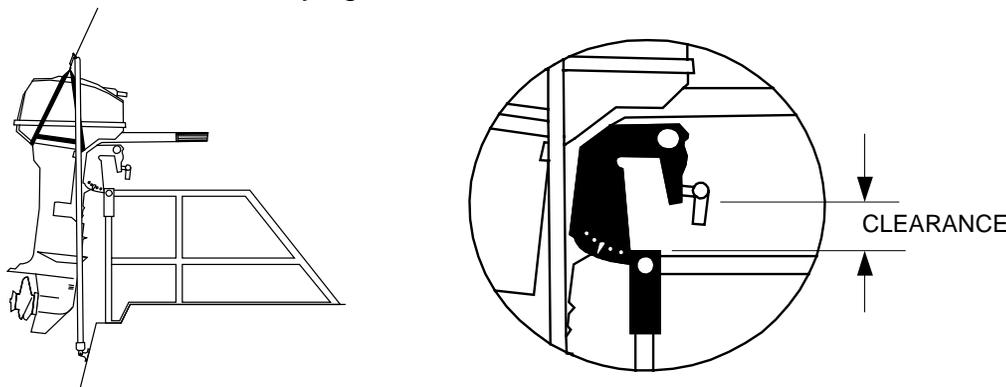
**TIP!** The frame is designed to be long enough for most applications. It may be shortened if you wish, simply by cutting the ends of the tubing with a hacksaw or pipe cutter. If you wish to shorten the frame we recommend that you do so only after having installed the deck hinges, tested the operation, and measured the excess clearance.
