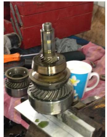
Once the assembly is inserted in the spline socket and you have tightened down the vice, place a wrench on the top nut (it is left handed). You may need to place the wrench handle into a pipe to get extra leverage to remove the nut. (I think a 27 ml socket fits)
