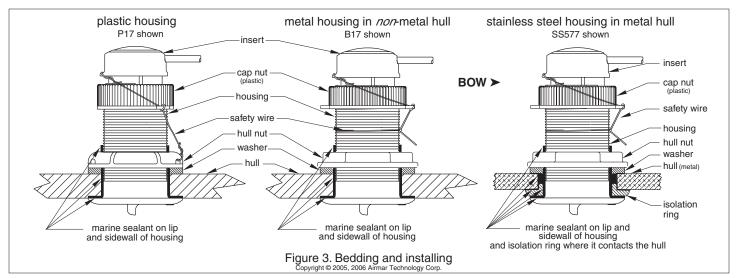
**Stainless steel housing in a metal hull**—To isolate the stainless steel housing from the metal hull, slide the isolation ring onto the housing. Apply *additional* sealant to the surfaces of the ring that will contact the hull, filling any cavities in and around the ring.
