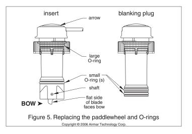
boat yards. O-rings *must* be free of abrasions and cuts to ensure a watertight seal. Order a replacement Paddlewheel Kit 33-398-04.
