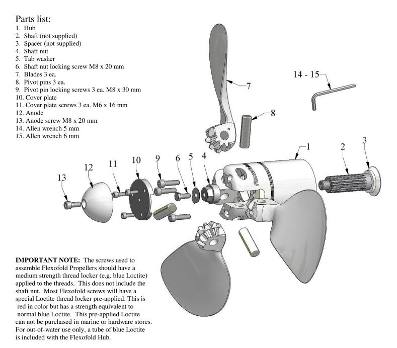
The screws with the pre-applied Loctite can be used for installations in or out of the water. Normal blue Loctite can only be used out of the water. If you remove a screw with the boat out of the water, the Loctite must be re-applied before re-using the screw. When changing or remounting a prop under water, you should first contact Flexofold to acquire a new screw set with the pre-applied Loctite.
