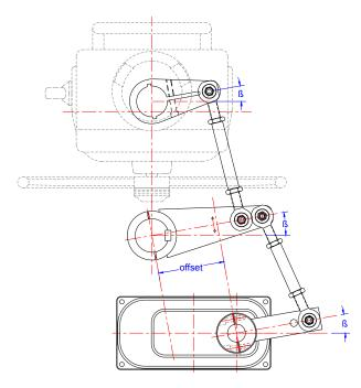
In principle the installation in combination with a rack and pinion system is the same as the standard installation except for the fact that the complete setup is rotated with the steering offset angle  $\beta$ .
