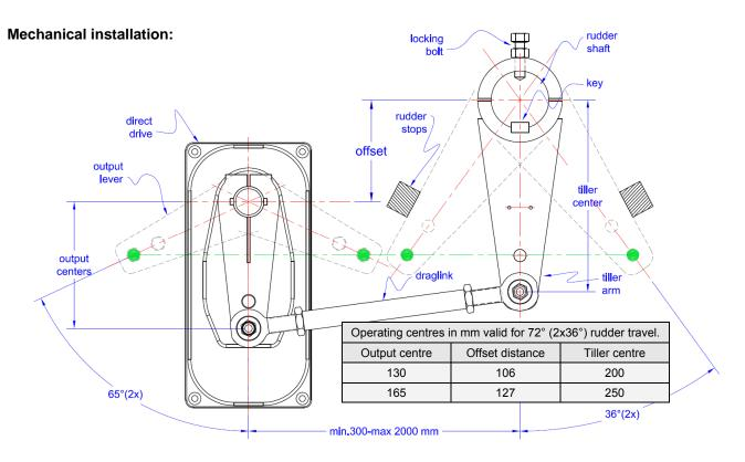
The direct drive uses "wide angle geometry". The result of this is 128° travel of the output lever and 72° travel of the tiller lever. To achieve an equal travel of the drive in port and starboard, the centre point of the output lever needs an offset to the rudderstock centre. The offset depends on the used lever centres. The above table shows the correct offset distances:
