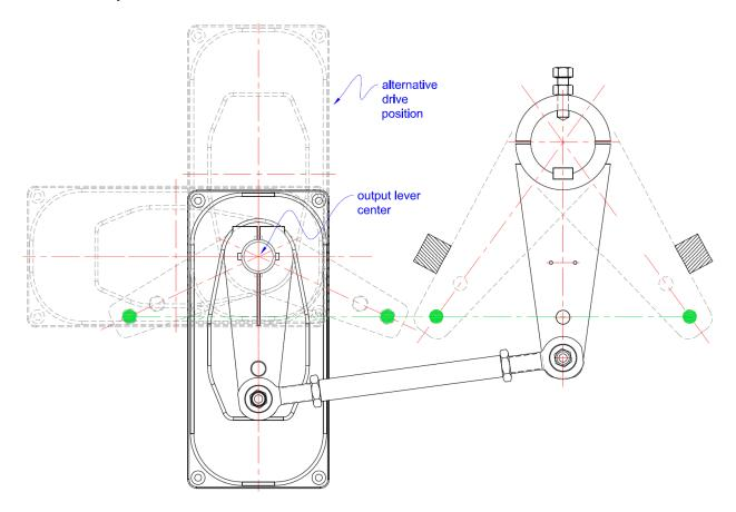
When another drive orientation is easier to install, one can rotate the drive motor in another direction, as long as the geometry between the center of the output lever and the rudder is kept the same,
