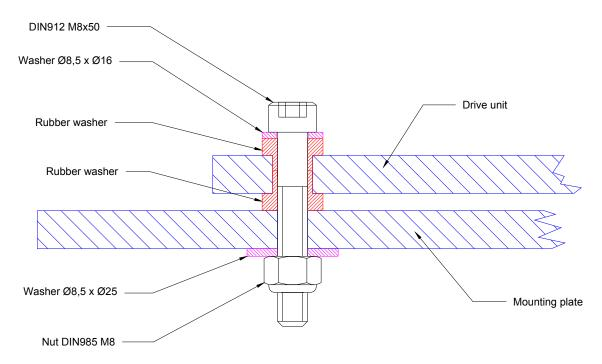
The vibrations from the autopilot drive motor and gears are often amplified multiple times by the deck or hull. This noise can be dramatically decreased by using the special bolts, rubber washers and bushes one can find in the bag supplied with the drive unit. When mounted like in the above illustration, the vibrations will be limited to the absolute minimum and a smooth and silent installation is guaranteed.
