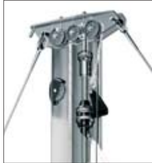
Seldén in-mast furling system: Geared line driver winch, tensioned luff extrusion, asymmetrical located sail slot and the patented load distributor of the halyard swivel. All to make furling an easy and fast operation.
