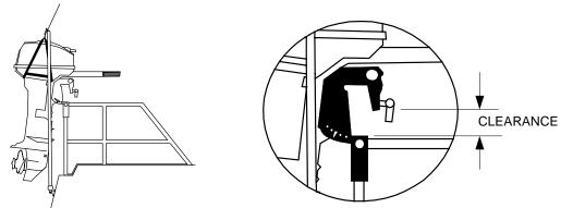
**TIP!** The frame is designed to be long enough for most applications. It may be shortened if you wish, simply by cutting the ends of the tubing with a hacksaw or pipe cutter. If you wish to shorten the frame we recommend that you do so only after having installed the deck hinges, tested the operation, and measured the excess clearance.
