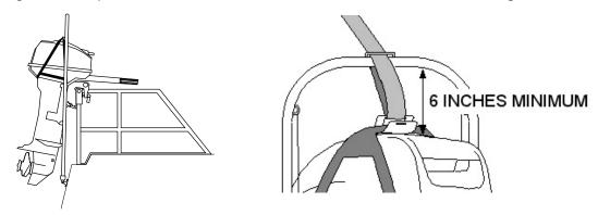
**IMPORTANT!** The frame must be mounted high enough to lift the motor clamp clear of the mounting bracket. This typically means leaving a MINIMUM of 6 inches from the bottom of the outboard carrying handle to the bottom of the frame.
