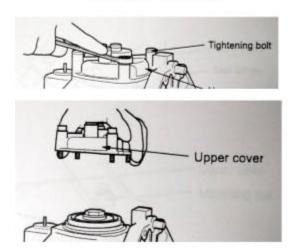
Figure 3: Step 1: Remove Upper Gear Tightening Bolts (4) And Upper Gear Cover
