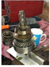
Once the assembly is inserted in the spline socket and you have tightened down the vice, place a wrench on the top nut (it is left handed). You may need to place the wrench handle into a pipe to get extra leverage to remove the nut. (I think a 27 ml socket fits)
