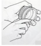
Figure 11: Step 7 Lapping Procedure For Drive Cone
