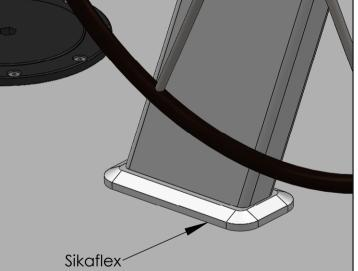
Before mounting the pedestal to the cockpit floor, it should be sealed with sikaflex.
