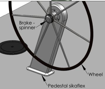
Dismount the brakespinner, then remove brass nut with 24mm wrench to dismount the wheel. Watch out for the key so you don't loose it.
